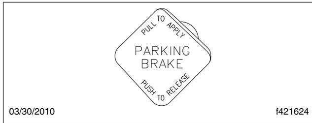
Fig. 5.1, Parking Brake Control Knob
